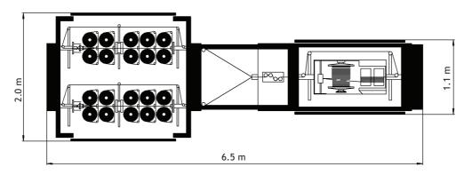
Motor power: 15 kW AC M55-3 weight: 4,600 kg M55-4 weight: 5,100 kg Height: 2.13 m
